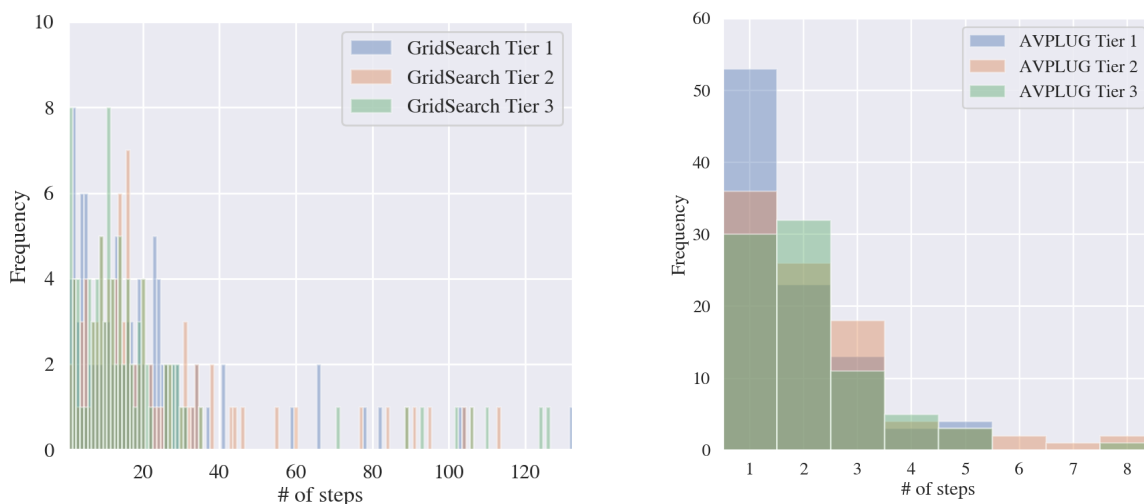
Figure 6.5: Comparisons of steps to completion of successful rollouts in simulation. The scale on the horizontal axis is 15\times larger for the GridSearch policy.
