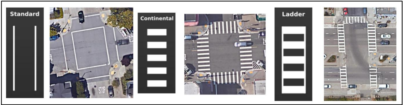
Figure 2a: Examples of three marked crosswalk categories in San Francisco visible from satellite imagery (top).
