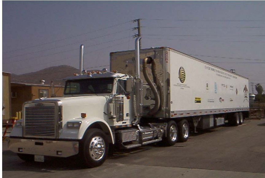
Figure 3.1. UCR’s Mobile Emissions Research Laboratory (MERL).
