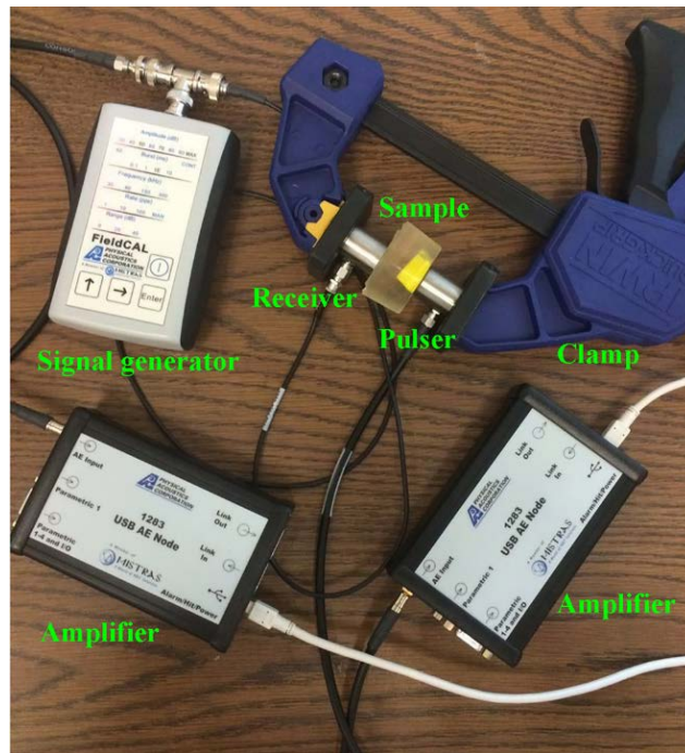
Fig. 10. Sound test on the sample. One transducer serves as the pulser and the other serves as the receiver. The incidence of a 30 kHz sine tone burst is generated by the signal generator.
