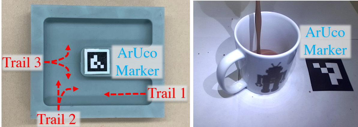
Figure 4.7. The left figure shows a top down view of the silicon cavity used for the Endoscopic Liquid dataset, and the liquid is injected with a syringe at the labelled points for three trials. The right figure shows a camera image from our Pouring Milk experiment set up.
