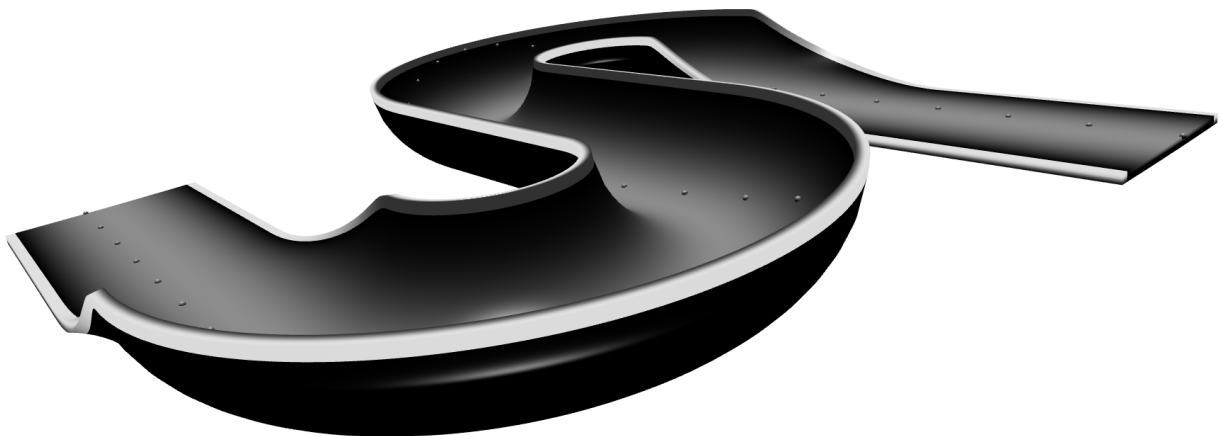
Figure 5.3: Raceline computed using a point mass model on the same non-Euclidean racetrack as Figure 5.2, with snapshots shown every tenth of a second. Dynamics were modeled by treating longitudinal and lateral forces as inputs, with a friction cone similar to the macroscopic limits on the dynamic vehicle model of Figure 5.2.
