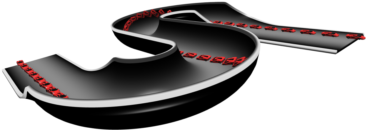
Figure 5.2: Raceline computed for a car on a non-Euclidean racetrack, with snapshots shown every tenth of a second. Vehicle dynamics were modeled with a two-track tire layout, combined-slip Pacejka tire model, and quasi-equilibrium weight distribution with the tangent contact road model. The 3D racecar asset was made by Sketchfab user Lexyc16, is licensed CC BY-NC 4.0, and can be downloaded from skfb.ly/opvyH
