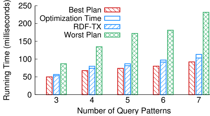
Figure 2.15: Query Execution Time of the best/worst plans, and the plan generated by SPARQL T optimizer for complex queries in Wikipedia
