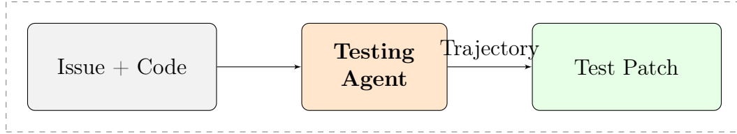
Figure 8.1: Execution-based verifier pipeline. A trained testing-agent ingests the issue and the current repository state and emits a single test_issue.py script with M = 10 diverse reproduction tests. These tests are then run against each candidate patch to compute the EB score.
