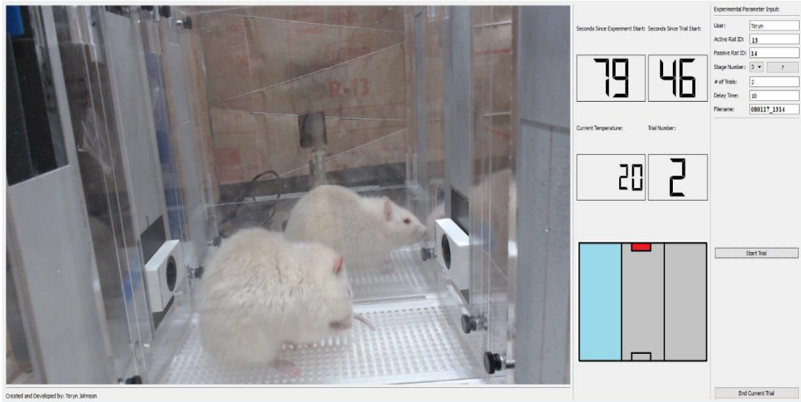
Figure 3. Depicts the graphical user interface used by the paradigm to feed the experimental timing, video live feed, temperature, trial number, and cartoon representation of the three chambers.
