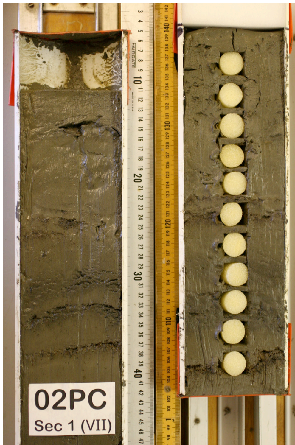
Figure 9. Photograph of the top piston core 02 (left) and its corresponding trigger core. Four POC layers can be identified in each core, indicating a correlation between the cores. It is evident that only ~5cm is missing from the top of the piston core (scale in cm).
