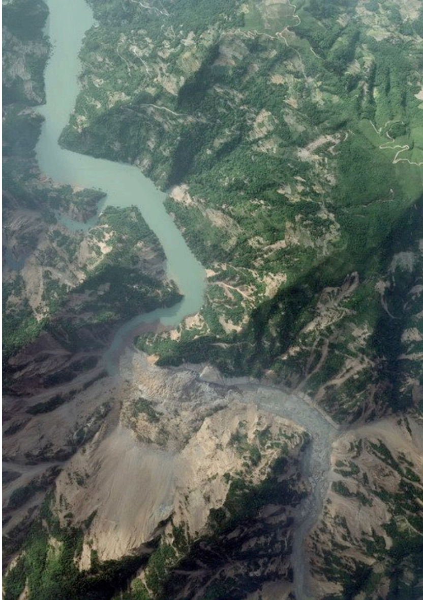
Figure 4. Sediment and biomass liberated from landslides are capable of filling channels and damming rivers. The landslide resulting from the Wenchuan, China earthquake of 2008 dammed the Jian River, creating Tangjiashan Lake, which had a volume of .128 km 3 .
