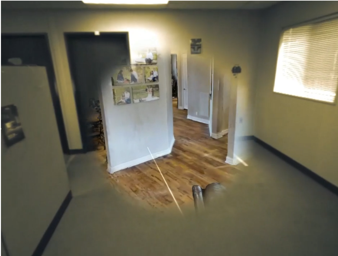
Figure 3.2: Blending in the real environment on the periphery to help users avoid physical obstacles. This technique was not used in our final walking experiment, but is an interesting option in smaller spaces.
