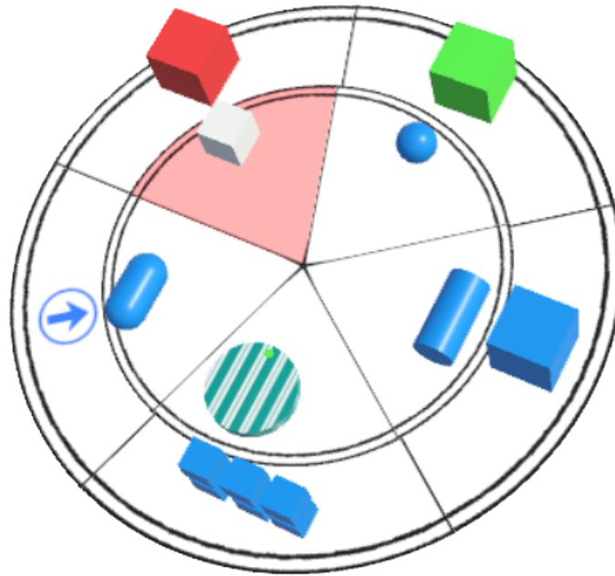
Figure 2.4: Our pie menu with some 3D geometry to showcase the functionality of each control. The menu appears above the touchpad on the controller.
