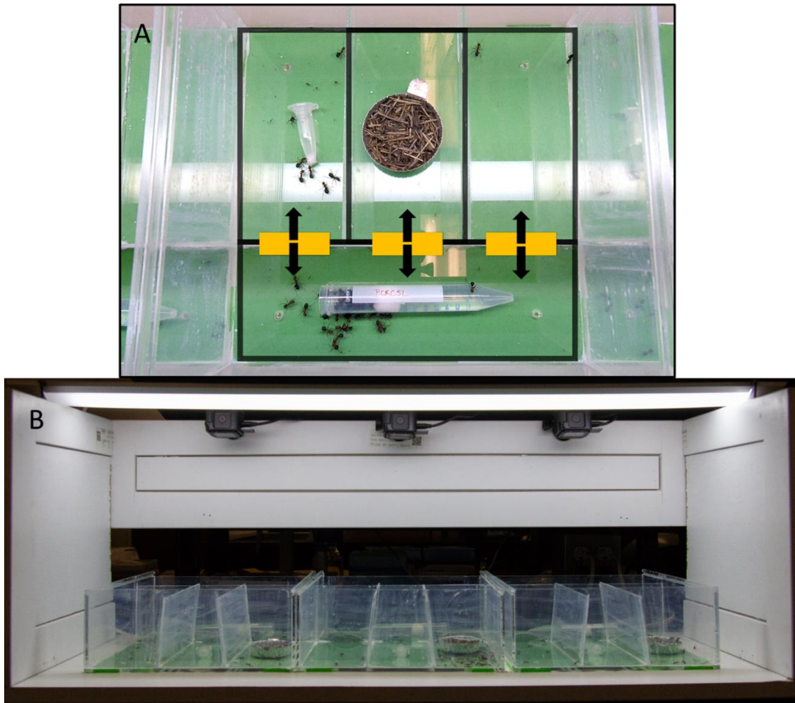
Figure 2.1: An example of our laboratory setup. A) A 23 x 23 x 10 cm compartmentalized artificial nest box. Compartments are outlined in black and passageways are indicated with yellow rectangles and black arrows. The nest box contains a 15 mL tube filled with water and plugged with cotton (bottom “nest” compartment), nest material in a weigh tray (upper middle “task” compartment), and sugar-water in a 1.5 mL tube with a cotton wick (upper left “task” compartment). B) Three artificial nest boxes containing different worker groups are shown side-by-side. Gopro™ Session 5 cameras were mounted directly above each nest box to collect video footage throughout each experimental trial.
