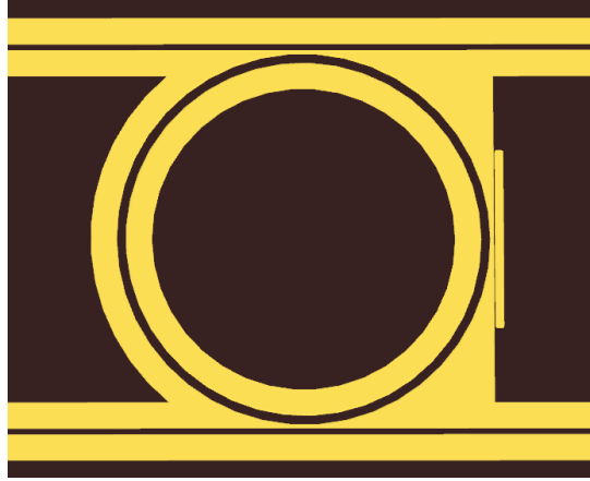
Figure 1.8: Schematic of an integrated optomechanical system, coupling a nanobeam to an optical ring resonator both fabricated from the same layer of \text{Si}_3\text{N}_4 .
