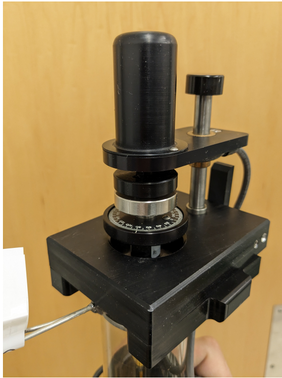
Figure 5.2: The rotator head containing stepper motor for insert.
