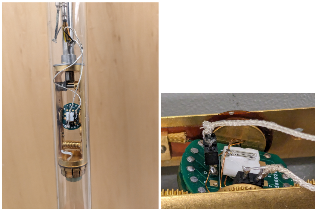
Figure 5.1: The PPMS Rotator Insert. Left: The PPMS rotator insert sample space with coaxial cables fed through. Right: The rotator sample space with tuning fork in qPlus configuration.
