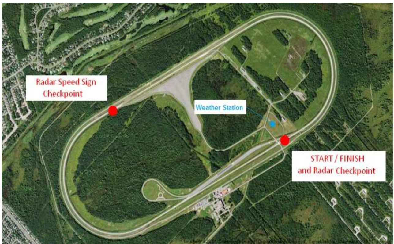
Figure 3-13. Map of test track with radar checkpoints and weather station location.
