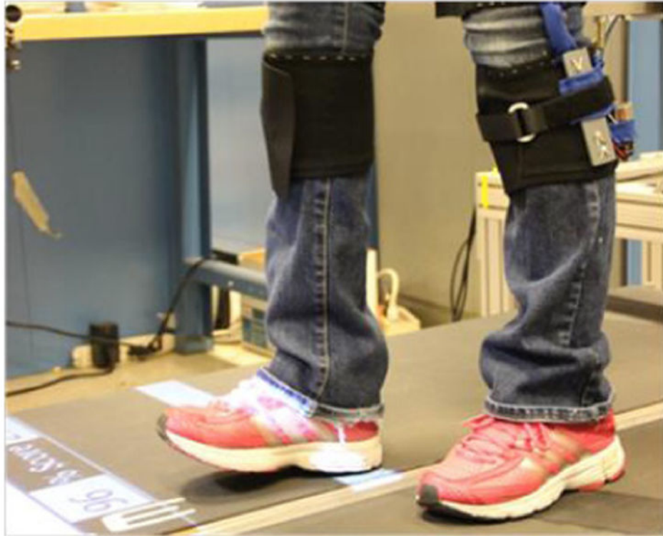
Fig. 8. Discrete training mode stepping. A target is shown (white bar). The participant locates the target position with the heel. The success rate can be seen in front of the participant to keep her engaged in the training session.
