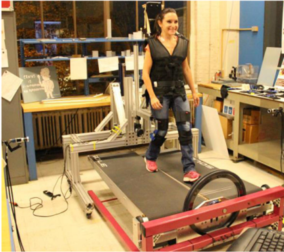
Fig. 1. A study participant with impairments due to Cerebral Palsy trains on the MIT-Skywalker. Subject is looking at a monitor that displays the training goals in a form of video-games.
