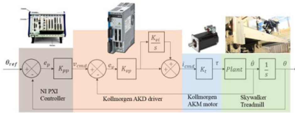
Fig. 5. Treadmill motion control loop.
