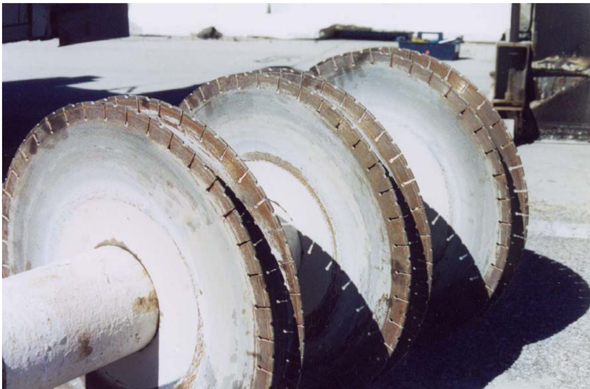
Figure 2.9. Removable saw blade arbor.
