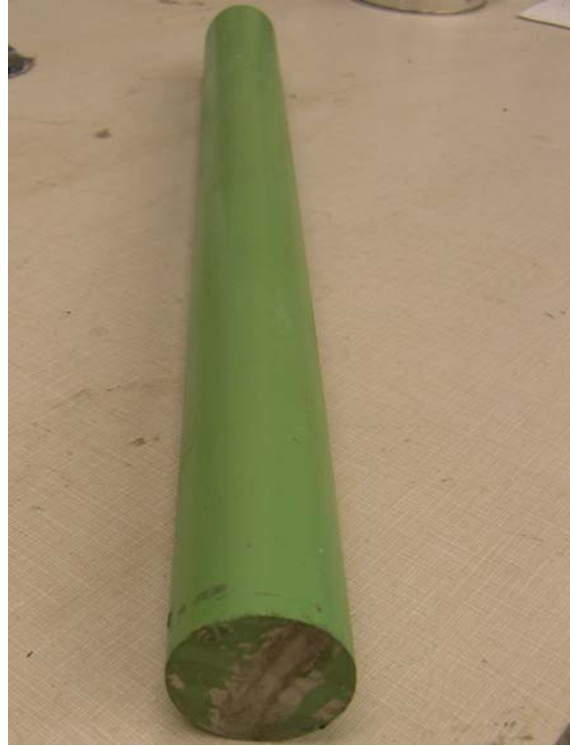
Figure 2.4. Epoxy-coated steel dowel.
