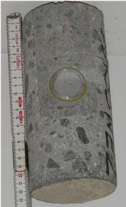
Figure 2.30. Core DBR33NE2 with hollow stainless steel dowel located 6 mm above mid-depth of slab.
