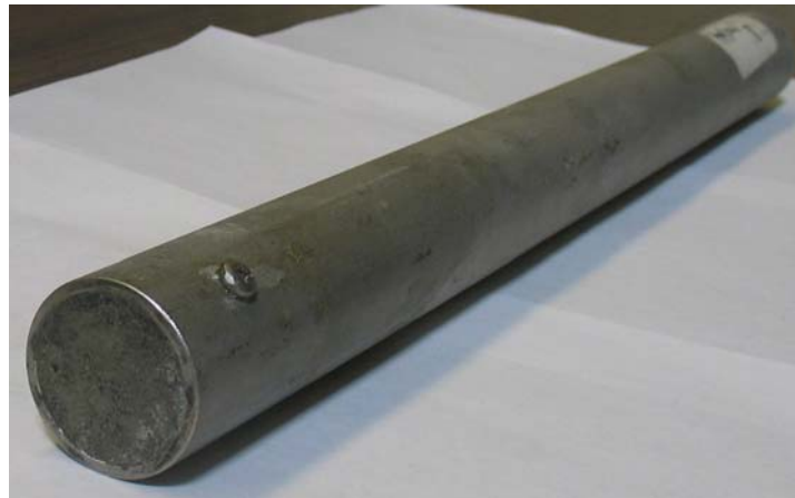
Figure 2.5. Hollow stainless steel dowel.
