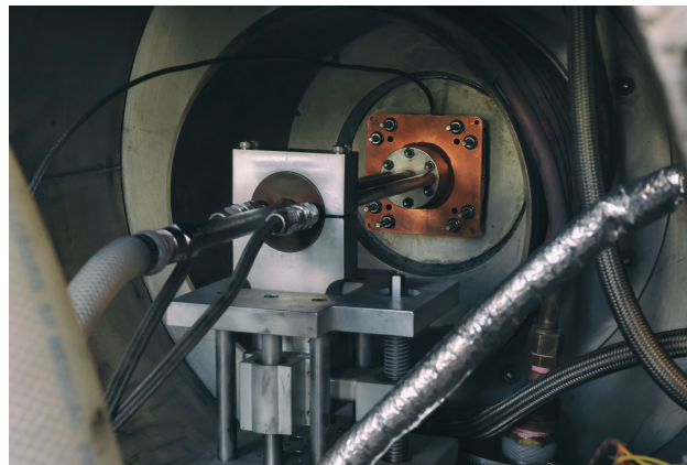
(b) Internal view. Sample positioned at 2.5 cm from jet outlet.
