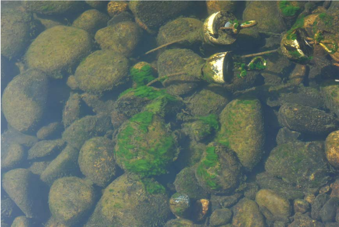
Figure F-1. Artificial redd at Site A on May 30, 2012. Coarse gravel and cobbles are present on the surface of this redd. No sand is visible on the artificial redd area. A piezometer cap is visible on the bottom of the photo and the sediment bag cable and floats are present above it. The piezometer cap is 5 cm in diameter.
