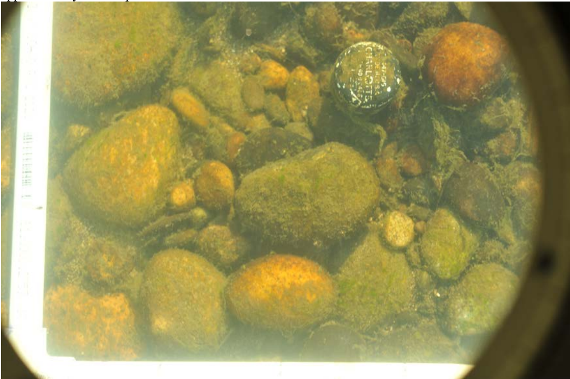
Figure F-3. Artificial Redd at Site C on May 31, 2012. A piezometer cap is shown in gravel with some signs of sand accumulation on the surface possibly indicating the backfill is approaching its capacity for accumulating sand. Piezometer cap is 5 cm in diameter.
