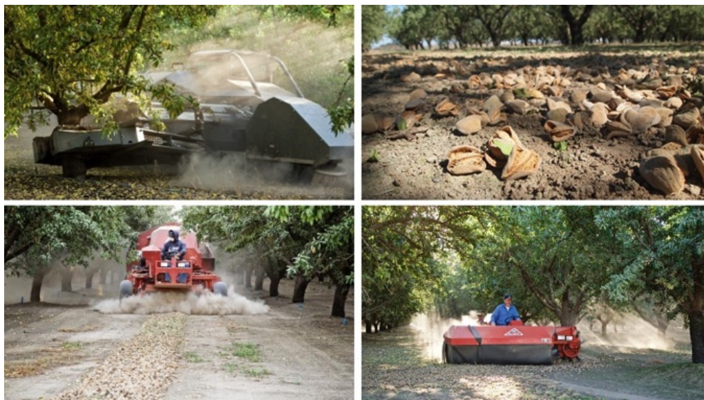
Figure 1.4 Conventional harvest of almonds. Clockwise from top left: shaking, on-ground drying, sweeping, and picking. (photos from Almond Board of California)
