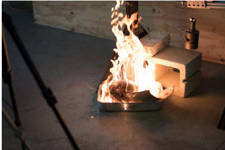
Figure 2.2 Ignited Fuel Bed After Experiment Using T-Slot Apparatus
