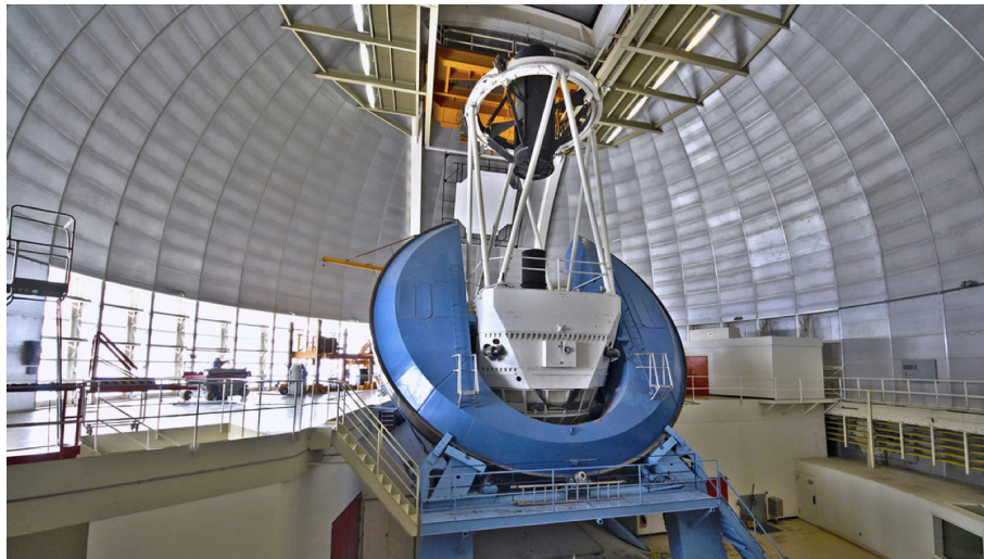
Figure 1.11: View of the 4m Mayall telescope from inside the dome. The primary mirror sits on an equatorial mount. The current mosaic corrector at the prime focus will be replaced for DESI.
