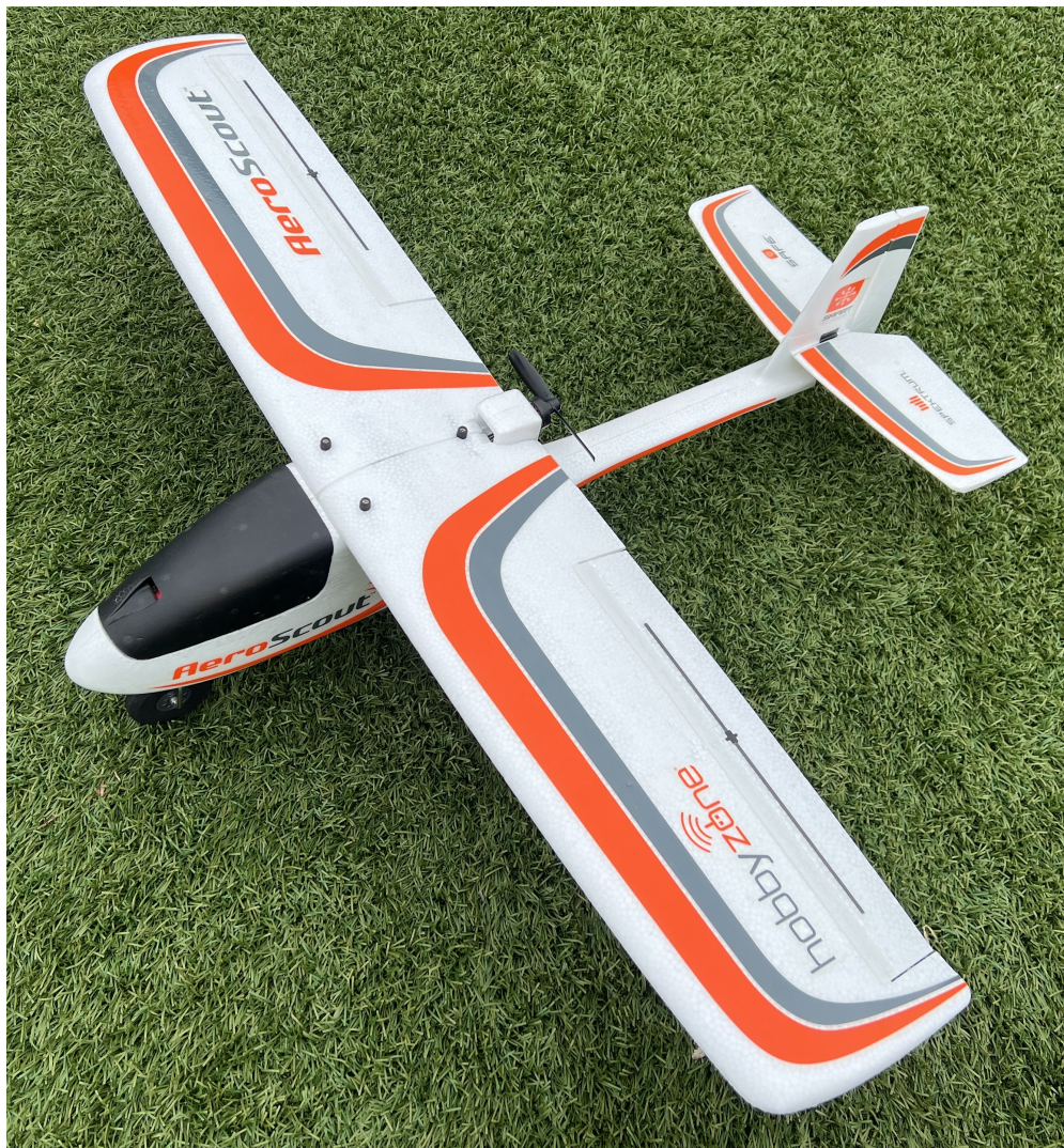
Figure 1.1: A radio controlled airplane with a span of 1.1 m .
