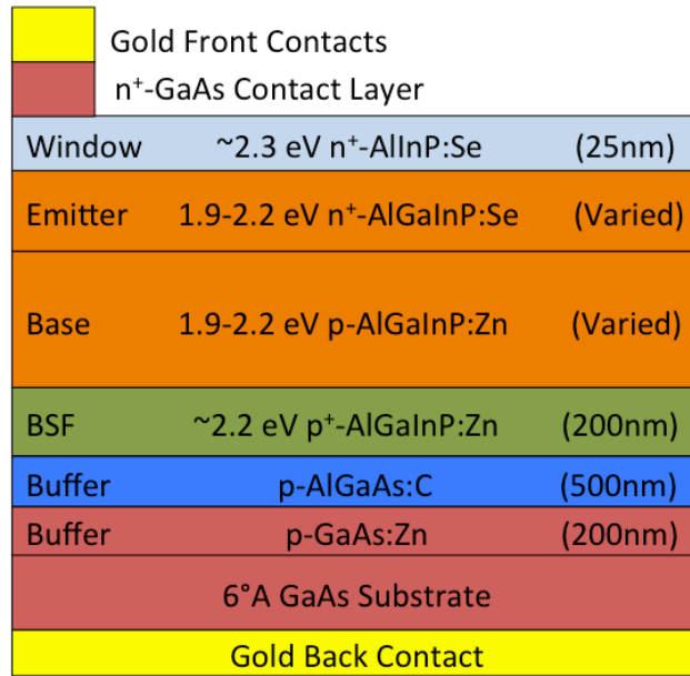
Figure 4.12: Schematic showing the structure of the epitaxially grown layers and metallization of the AlGaInP solar cells studied in this work. The diagram is not to scale [120].
