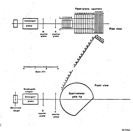
Fig. 6. The broad-range magnetic spectrometer and counter array.
