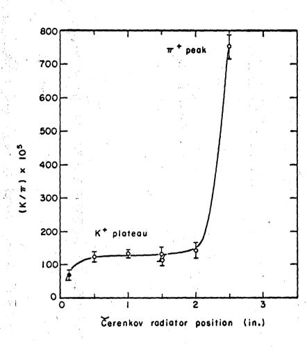
Fig. 4. Counting rate in Cerenkov counter versus radiator position. K<sup>+</sup> mesons were selected by fixing the radiator at the center of the plateau in this curve.
