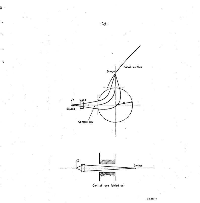
Fig. 7. Illustration of focal properties of spectrometer.
