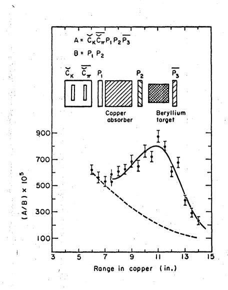
Fig. 9.  $K^{\dagger}$  stopping rate as function of degrader thickness.
