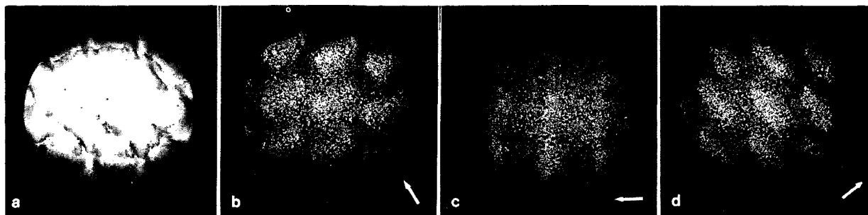
Fig. 2. Optical analysis of contrast variation of paraffin lattice images, within small exposed areas. In this example the illumination spot size had a diameter of 2000 Å. (a) Bright-field image of the electron micrograph obtained on a coherent-optical reconstruction bench. (b,c,d) Dark-field images of the micrograph obtained by masking out all but one of the diffraction spots in the optical transform of the micrograph. Arrows indicate the direction of the reciprocal lattice vector associated with the diffraction spot used to form each image.
