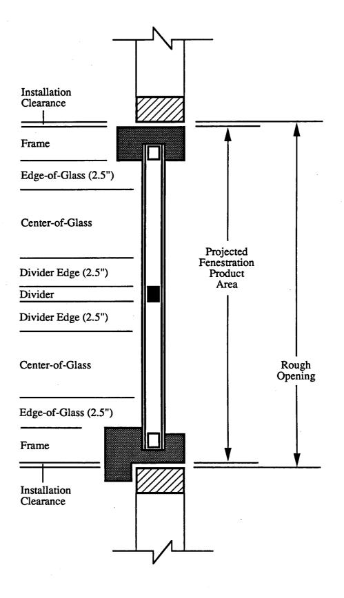
Figure 4: Window Components in Section
