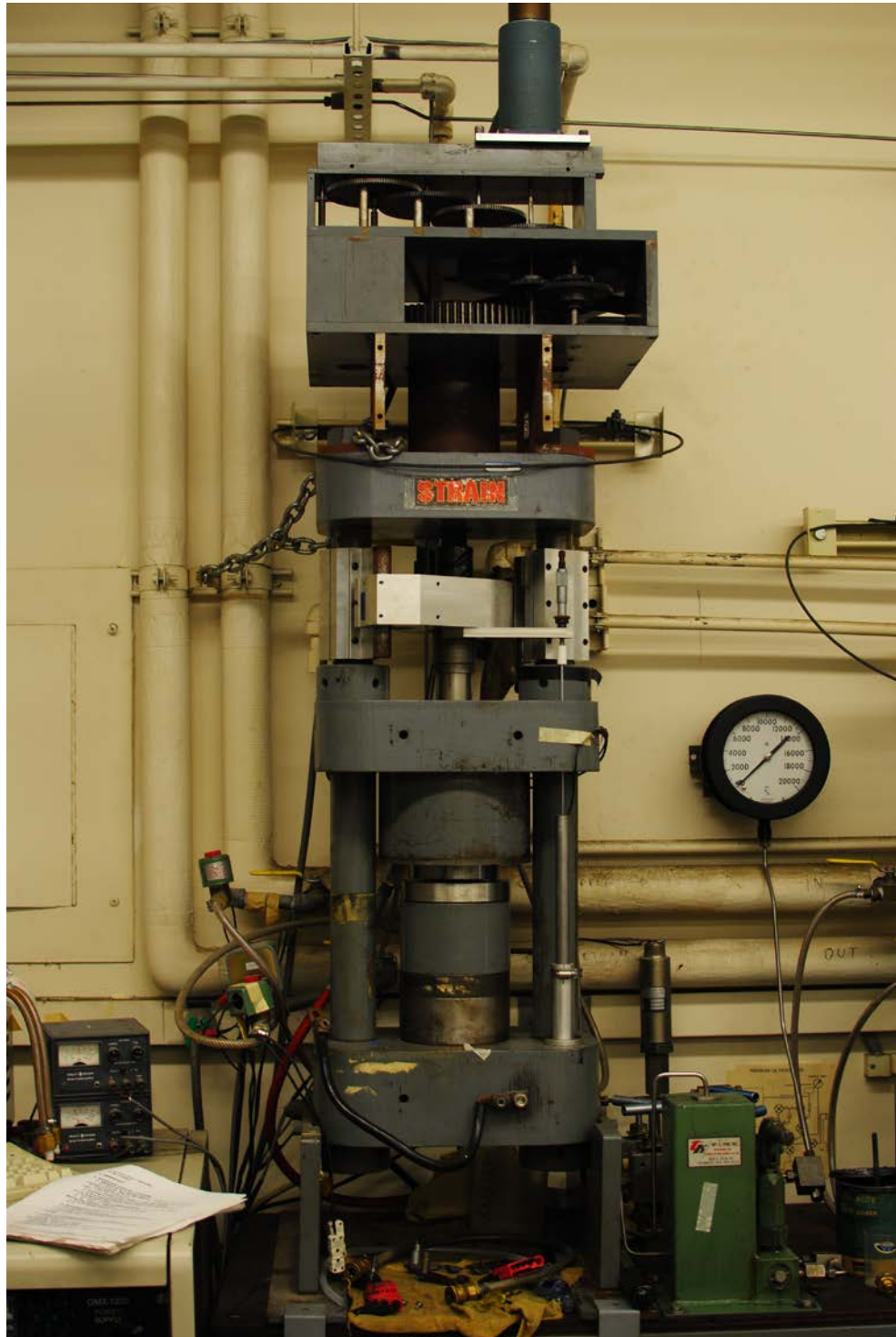
Figure 1.1 Photograph of Rig-2 Griggs apparatus in the Tectonophysics Laboratory at University of California, Riverside.
