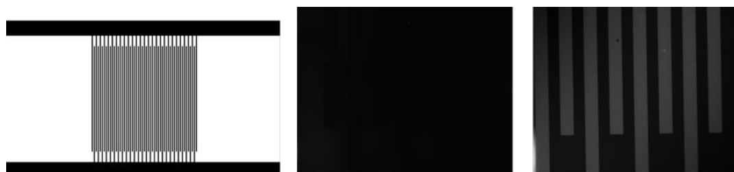
Figure 46: (left) CAD diagram of the interweaving 50um thick gold electrodes. Electrodes images under a fluorescence microscope (center) before and (right) after functionalization of BODIPY die to confirm MUA-EDC-NHSS-Lys-Peptide bond. Each gold lines are 50 \mu\text{m} in width.
