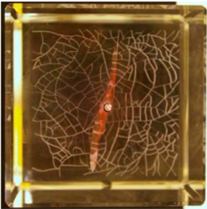
Fig. 13. A comparison between a) the simulated fracture trace within the pre-existing fractures and b) the visualization of hydraulic fractures in the laboratory test.
