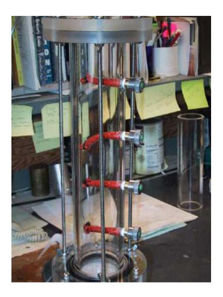
Figure 2.4: Photograph showing the assembly used to extract gas samples from within the column. The gas permeation samplers were constructed of silicon tubing (red), inserted through the column wall, and connected to barbed gas chrom atograph septa valves (m etal/green). Gas diffused from the column through the tubing and was withdrawn by syringe.
