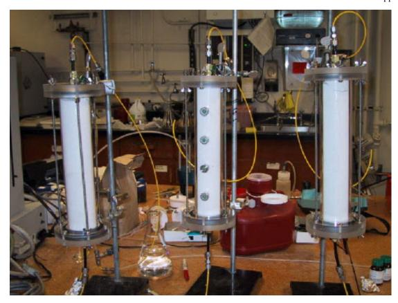
Figure 2.1: Photograph show ing three of the columns used in the experiment and the general design of each. The features shared by all of the columns are clear Polycarbonate chambers, gas and water tight seals, removable end caps, and adjustable influent and effluent lines.
