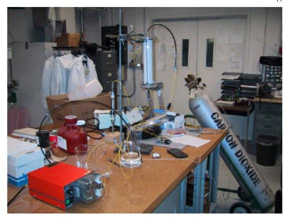
Figure 2.2: Photograph showing the general arrangement of the carbon dioxide flushing system. Gas flowed from the cylinder through a calibrated flow indicator (mounted on the ring stand to the lower left of the column) and upward through the column displacing the less dense ambient pore space air.
