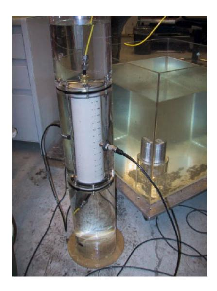
Figure 2.5: Photograph showing the apparatus designed to make acoustic wave measurements. The sediment column was inserted into a water-filled tube into which the acoustic transducers were coupled. The transducers (piezoelectric cylinders with black connecting cables) remain fixed while the column was raised/lowered within the tube (measurement locations are visible).
