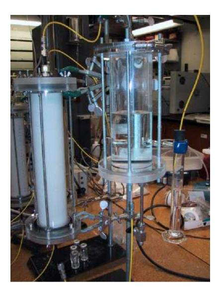
Figure 2.3: Photograph showing the assembly used to make measurements of saturated hydraulic conductivity. Note the modified Mariotte bottle mounted on the ring stand above and to the right of the column. The  $\Delta h$  value is determined by measuring the distance from the bubble tube (inside the fluid reservoir) to the outflow (inside the graduated cylinder).
