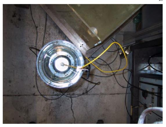
Figure 2.6: Photograph showing the apparatus designed to make acoustic wave measurements from the top. The  $180^{\circ}$  alignment of the transducers is visible as is their offset from the column wall.
