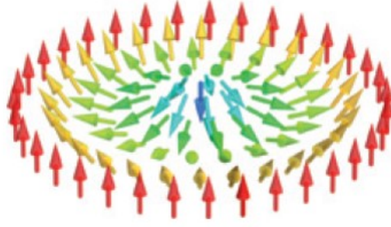
Figure 5.1: Representation of the magnetic configuration in a skyrmion as described in the reference [70].
