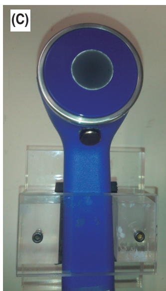
Figure 8. Setup for acoustic characterization. A) Pulse–echo setup using a contact transducer. B) Setup to measure the acoustic field in water with needle hydrophone. C) Photograph of commercial ultrasound transducer with an 8YSZ sample attached to the radiating surface; the sample did not cover the entire surface.
