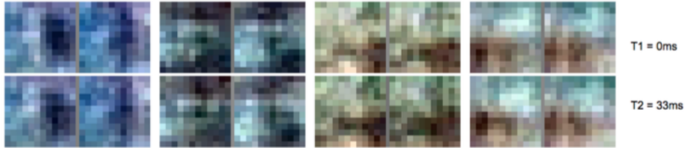
Figure 2.2: Gradient Ascent Visualizations. Shown are four neurons’ receptive fields from Layer 1 of our first self-driving network. Each neuron filter is divided into sub-filters, with one sub-filter per camera, per input frame – hence the 2x2 layout per neuron filter. These filters are appear sensitive to optical flow and stereoscopic disparity.
