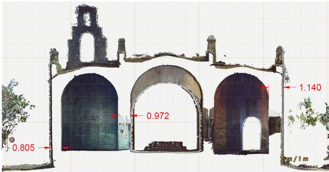
Figure 6.3 Section cut of the church data: Example dimensions are shown to illustrate the precision and utility of TLS.
