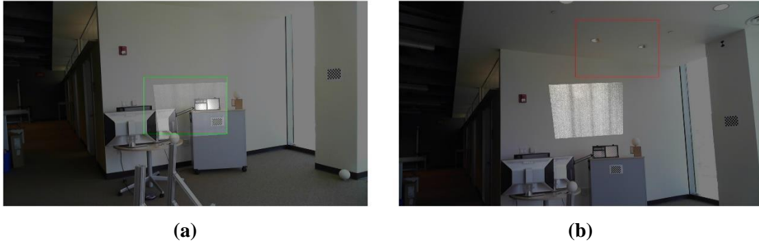
Figure 5.6 Multimodal registration attempts using mutual information (a) Success with features and (b) Failure with no common features.
