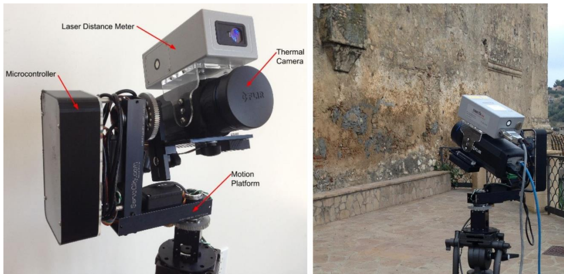
Figure 4.2 Annotated APT instrument (left) and the APT instrument deployed in the field (right).
