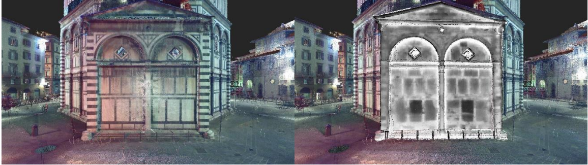
Figure 7.8 Information model of the Baptistery showing the toggling of the thermal layer.
