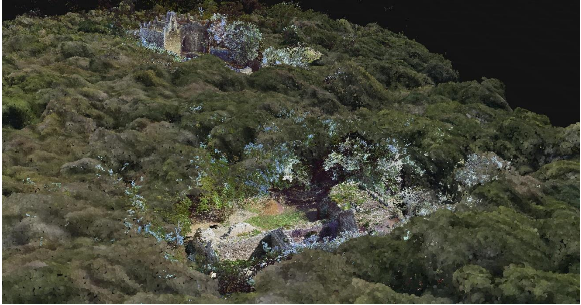
Figure 6.1 Aerial view of the integrated data set from the site of Ecab combining TLS, ground based SfM, and aerial SfM.
