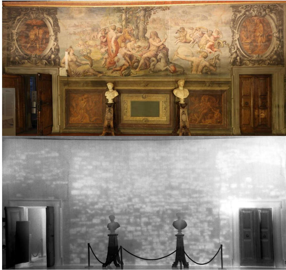
Figure 7.3 High-resolution thermal and visible layers of the Room of the Elements' West wall.
