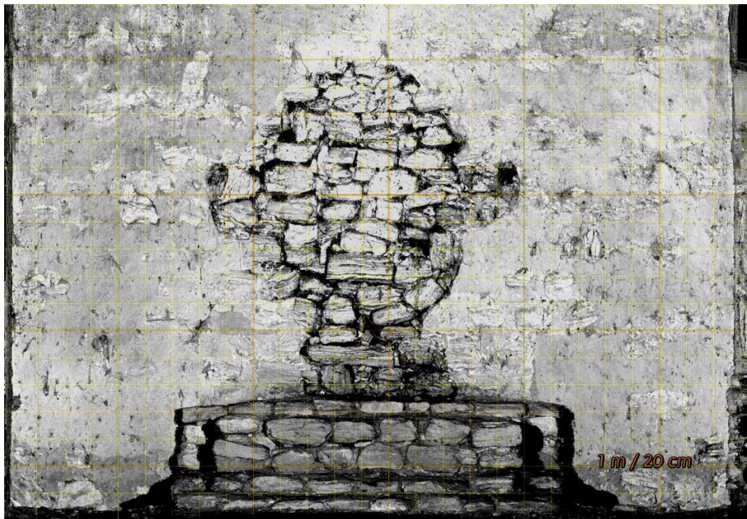
Figure 6.4 Orthogonal image from the grayscale laser scanning point cloud outlining the vandalism of the church's altar.
