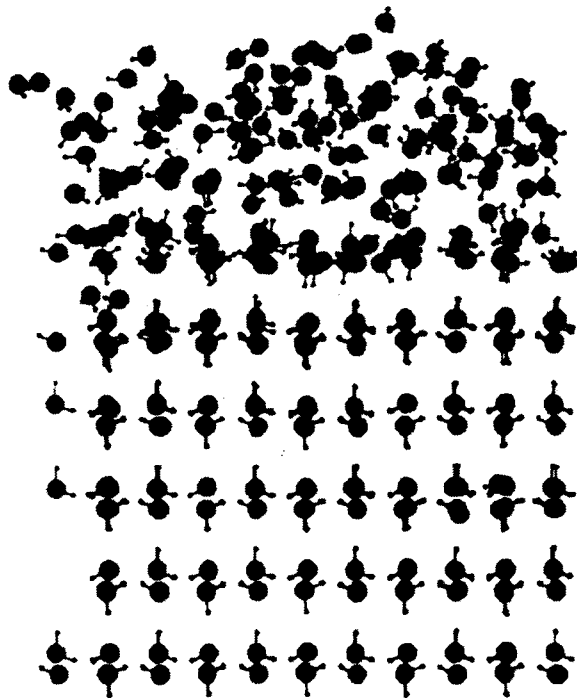
Figure 2.3: Molecular dynamics simulation of the (0001) basal surface of ice I h at 265 K (from Ref. [24]).
