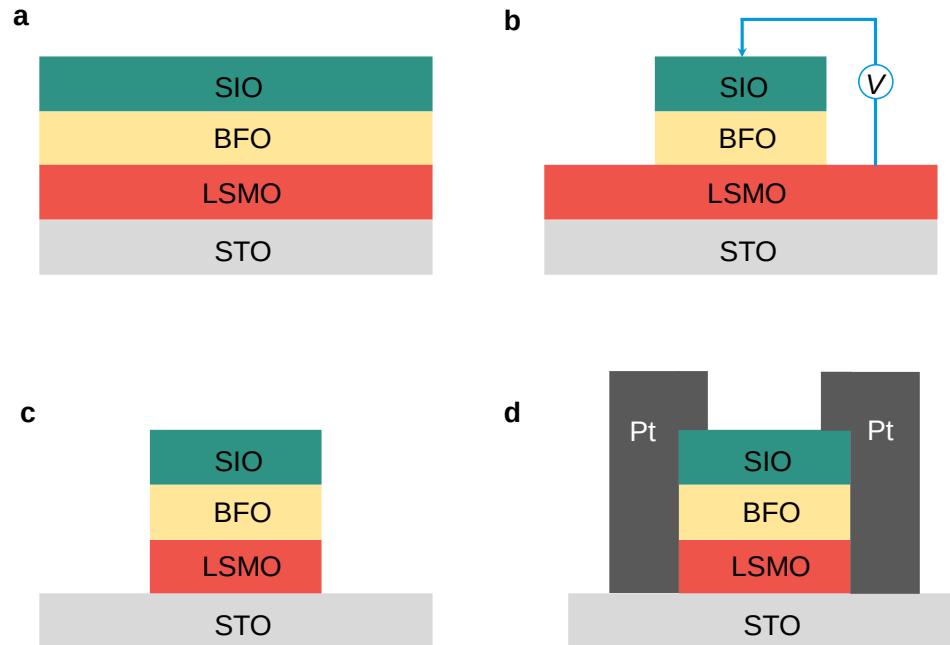
Figure 5.1: General device fabrication process for polarization dependent spin transmission study. a , The tri-layer heterostructure consists of LSMO, BFO, and SIO. b , Ferroelectric switching configuration. V : voltage applied. c , The heterostructure before electrode deposit. d , The profile of the device for spin transmission study.
