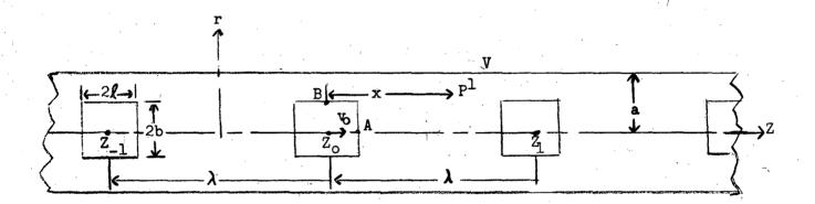
We assume that the bunches are identical and extend infinitely in both directions. The separation of their centers is  $\lambda$ , the radius is b and the length 2. The common velocity is  $v_0$  the charge density  $\rho$ . If
