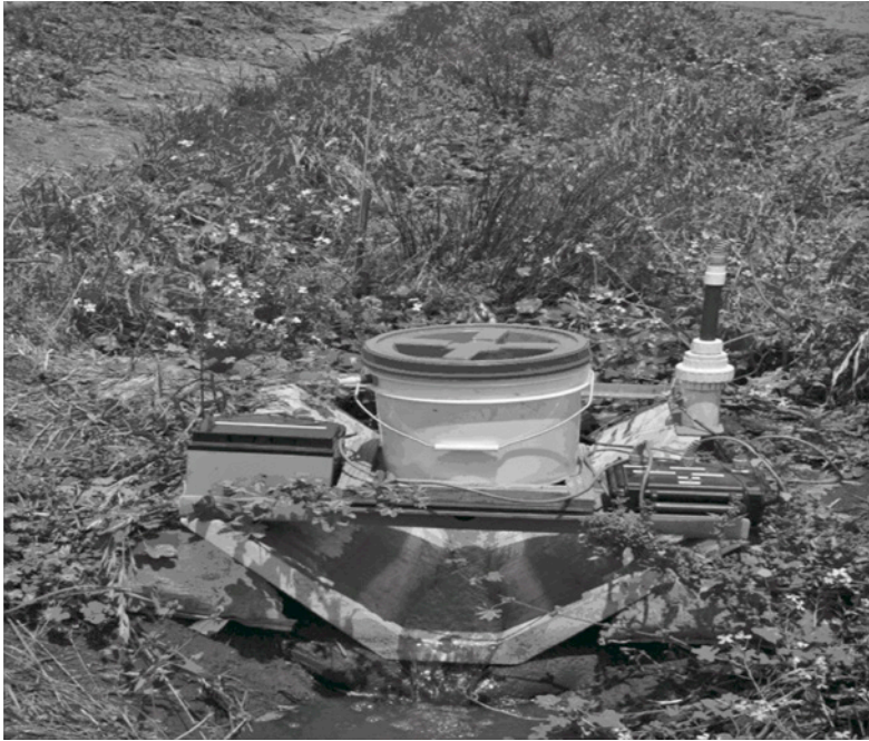
Figure 14. Anderson trial showing vegetated ditch and electronic dosing unit, 2008. Photo by B. Anderson
