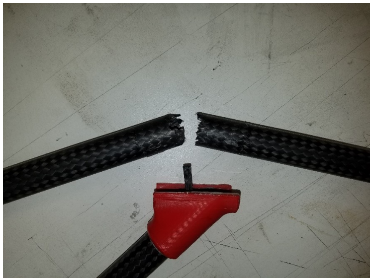
Figure 3.6: Frame Arm Appendage Structural Failure
