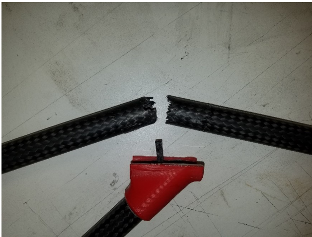
Figure 4.6: Frame Arm Appendage Structural Failure
