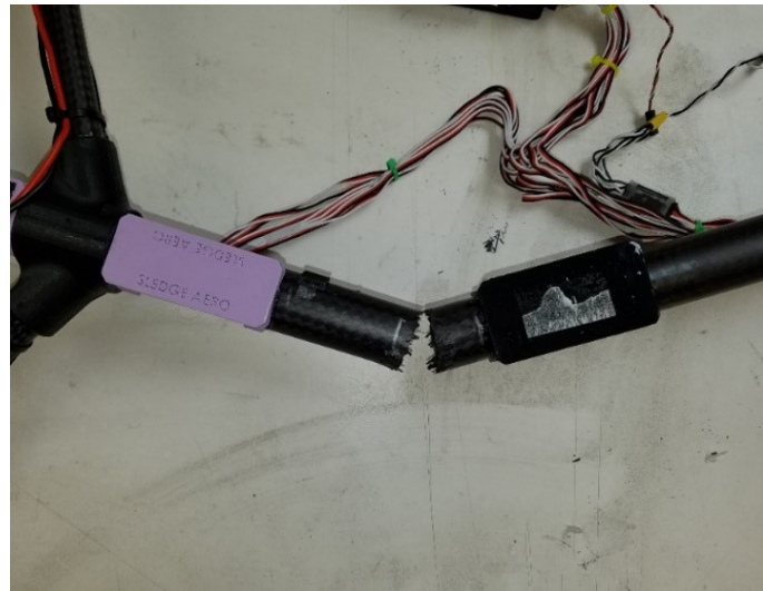
Figure 3.14: Fuselage Frame Structural Failure
