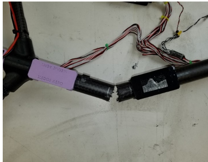
Figure 4.11: Fuselage Frame Structural Failure
