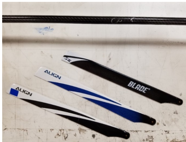
(b) Rotor Blade Comparison, from Top to Bottom: OEM Blade, Align Blade (blue), Align Blade (black)
