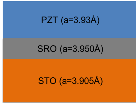
Figure 2.7. The cross section of PLD grown PZT film on STO substrate.
