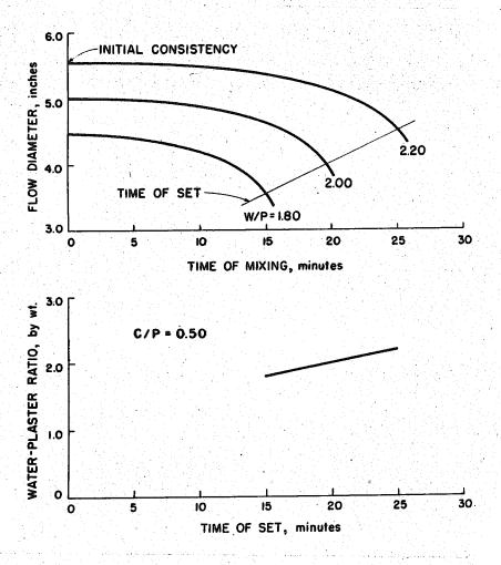
FIGURE 57 - EFFECT OF WATER ON CONSISTENCY AND SET
