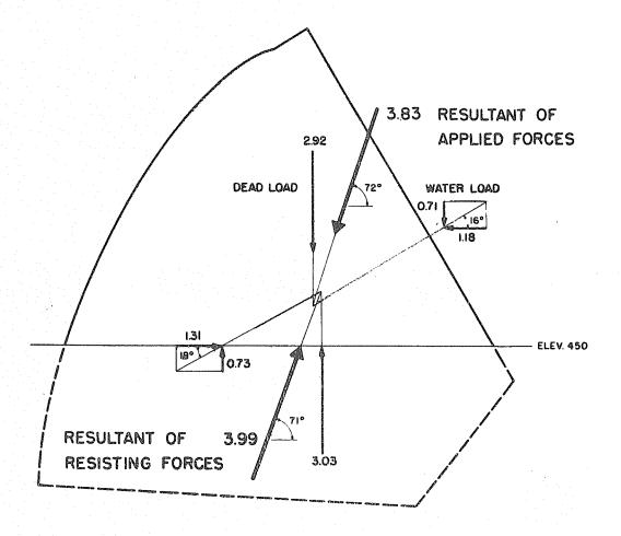
FIGURE 40 - COMPARISON OF RESULTANT OBSERVED RESISTING FORCES WITH RESULTANT COMPUTED LIVE AND DEAD LOADS
