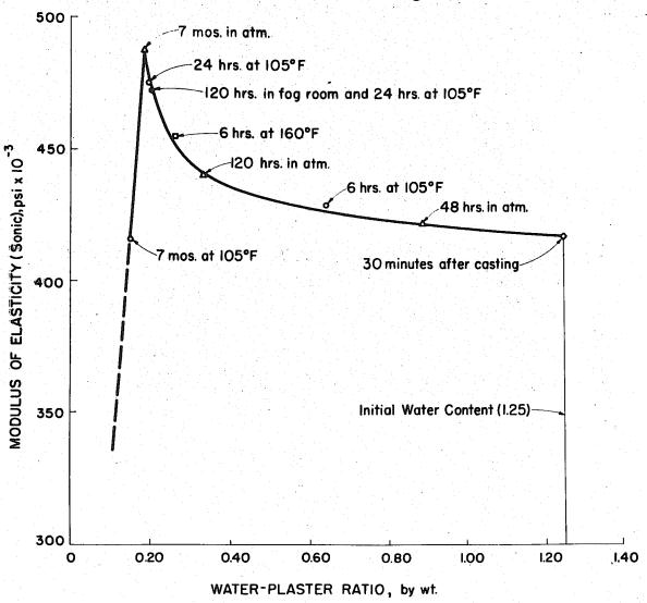
FIGURE 55 - EFFECT OF DRYING ON ELASTICITY
