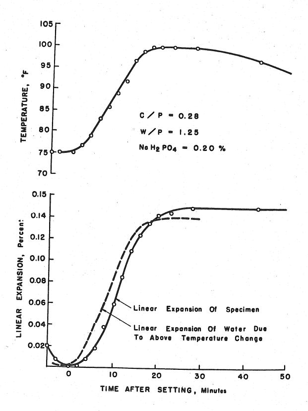
FIGURE 63 - TIME, TEMPERATURE AND VOLUMETRIC RELATIONSHIPS DURING HYDRATION OF PLASTER
