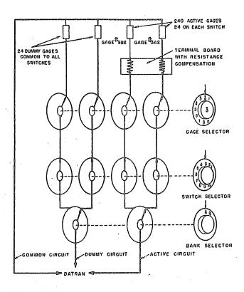
FIGURE 18 - SWITCHING CIRCUITS
