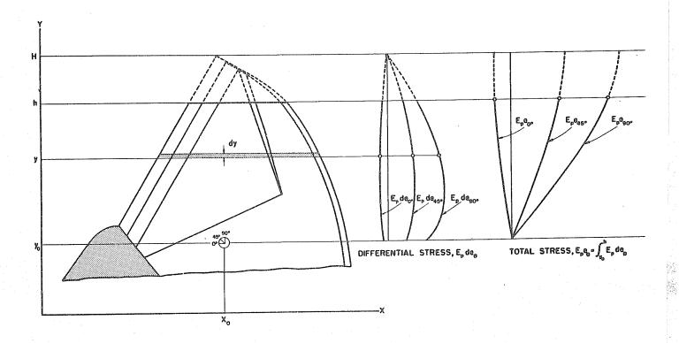
FIGURE 28 - NOTATION FOR METHOD OF INTEGRATION FOR DEAD LOAD STRESSES
