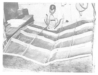
B - FITTING BALSA STIFFENER CORES ON FIBERGLAS MOLD
