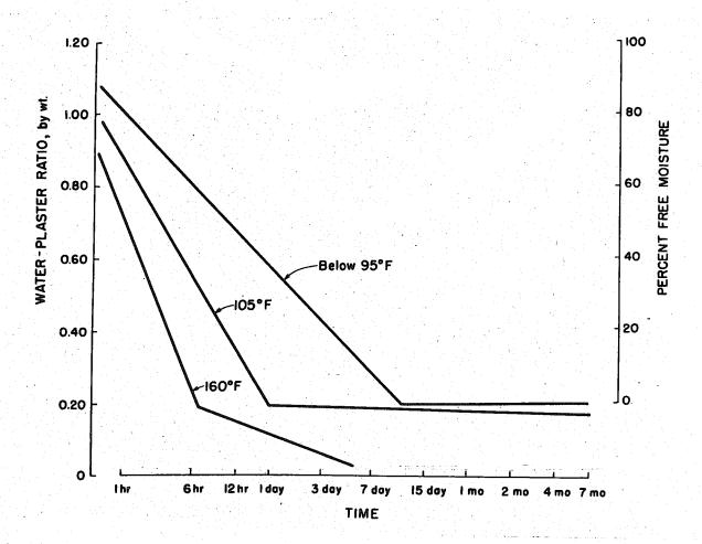
FIGURE 56 - DRYING RATES AT VARIOUS STORAGE TEMPERATURES
