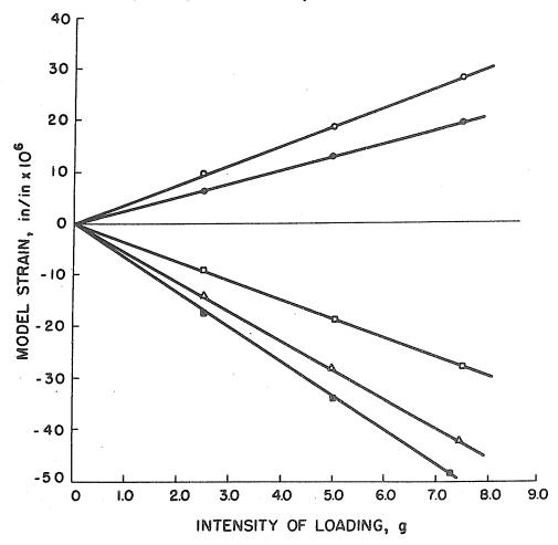
FIGURE 22 - LINEARITY OF RESPONSE OF MODEL TO INTENSITY OF LOAD
