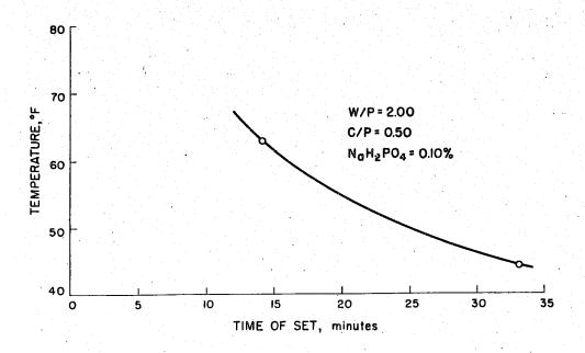
FIGURE 60 - EFFECT OF TEMPERATURE ON TIME OF SET
