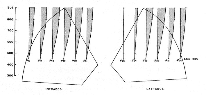
A - VERTICAL STRESS AT ELEVATION 450
