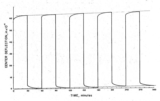
FIGURE 65 - EFFECT OF REPEATED LOADING ON FLEXURAL CREEP
