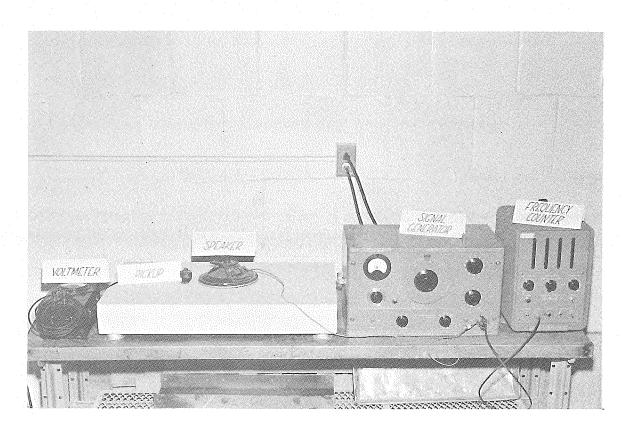
FIGURE 48 - APPARATUS FOR DETERMINING MODULUS OF ELASTICITY
