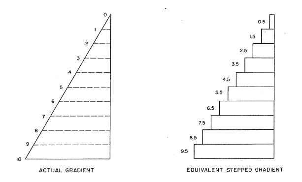
FIGURE 10 - ACTUAL HYDROSTATIC PRESSURE GRADIENT AND EQUIVALENT STEPPED GRADIENT
