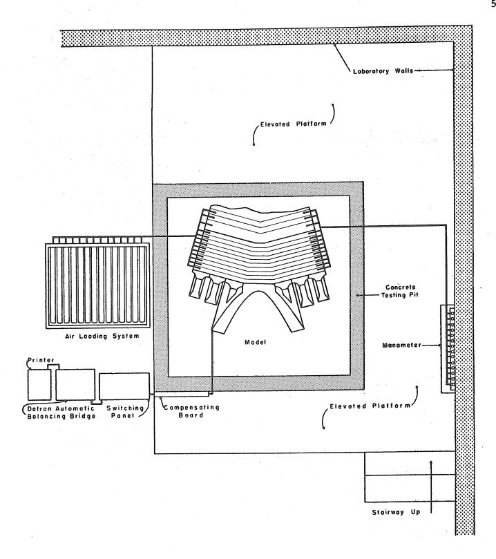
FIGURE 21 - LOADING AND INSTRUMENTATION FOR HYDROSTATIC LOAD TESTS
