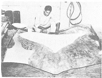
B - THE COMPLETED PROTO-TYPE PLUG IN PLACE ON PROTOTYPE FOUNDATION SURFACED WITH PLASTER, WITH SPRUES ADDED
