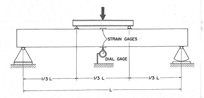
FIGURE 46 - SET UP FOR DETERMINING FLEXURAL MODULUS OF ELASTICITY
