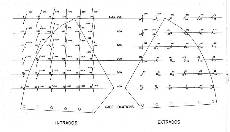
FIGURE 32 - PRINCIPAL STRESSES AT BASE DUE TO DEAD LOAD AT VARIOUS STAGES OF CONSTRUCTION
