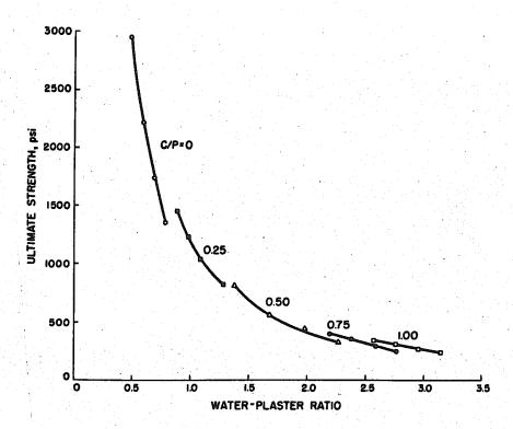
FIGURE 51 - EFFECT OF WATER-PLASTER RATIO ON COMPRESSIVE STRENGTH
