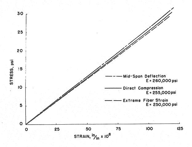
FIGURE 47 - STRESS-STRAIN DIAGRAMS FOR THREE TYPES OF TEST FOR MODULUS OF ELASTICITY
