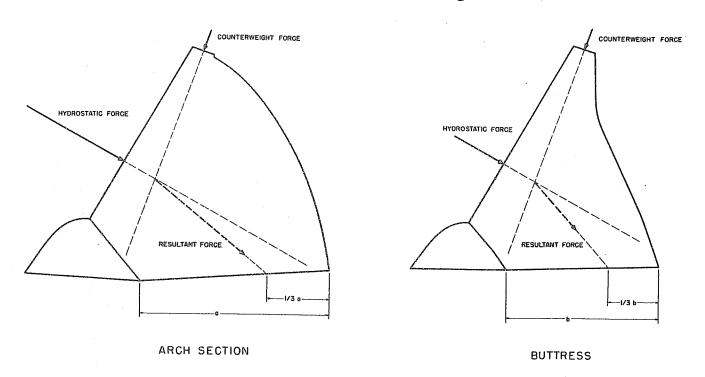
FIGURE 14 - EFFECT OF COUNTER WEIGHT FORCES ON STABILITY
