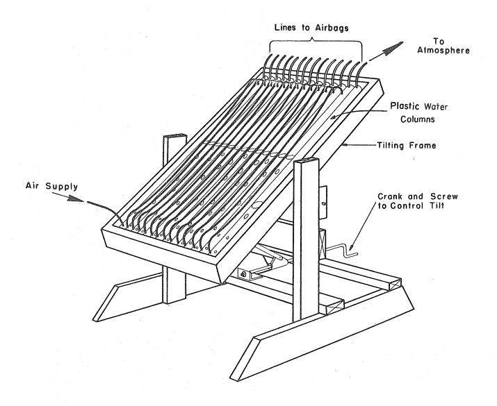
FIGURE 11 - SKETCH OF DIFFERENTIAL PRESSURE CONTROLLER
