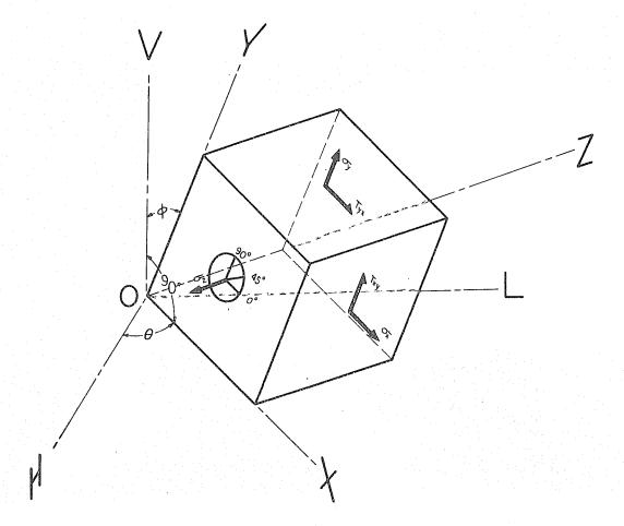
FIGURE 38 - ELEMENT FOR TRANSFORMATION OF SURFACE STRESSES
