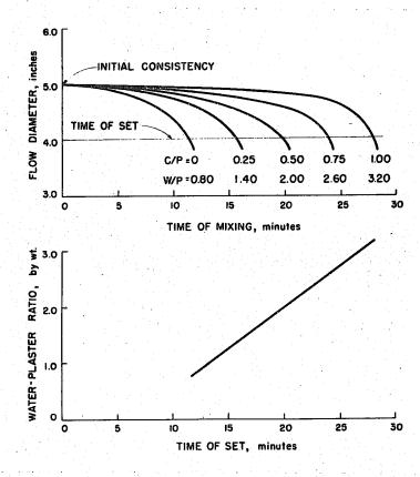
FIGURE 59 - EFFECT OF WATER AND CELITE ON TIME OF SET
