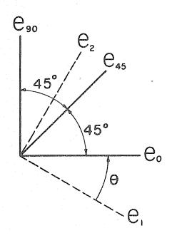
FIGURE 24 - ORIENTATION OF PRINCIPAL STRESSES
