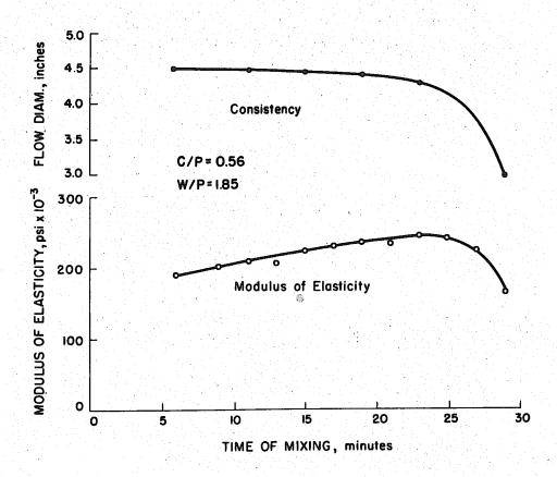
FIGURE 64 - EFFECT OF MIXING TIME ON CONSISTENCY AND MODULUS OF ELASTICITY
