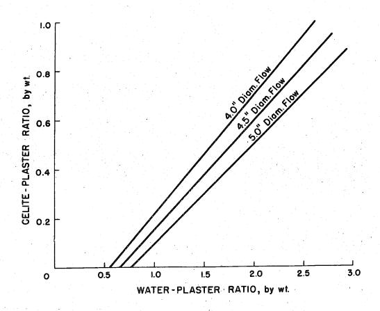
FIGURE 58 - EFFECT OF CELITE ON CONSISTENCY
