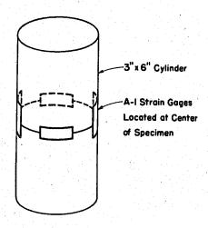
FIGURE 53 - MEASUREMENT OF POISSON'S RATIO USING SR4 GAGES
