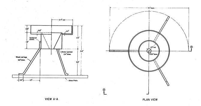
FIGURE 42 - DETAILS OF CONSISTOMETER
