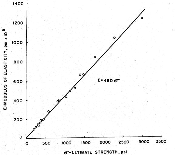
FIGURE 52 - RELATION BETWEEN ELASTIC MODULUS AND STRENGTH OF PLASTER
