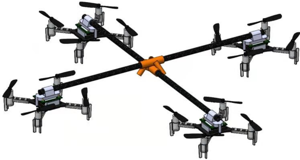
Figure 5.5: The CAD model of the proposed aerial platform, which is utilized to construct physical model with Simulink SimScape toolbox.
