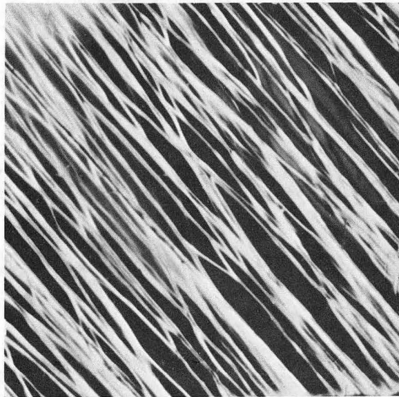
FIG. 8e SLIP TRACES OF SPECIMEN (A2S) DEFORMED AT 550°K TO 5% ELONGATION. \chi'_2 = -30^\circ "A"
