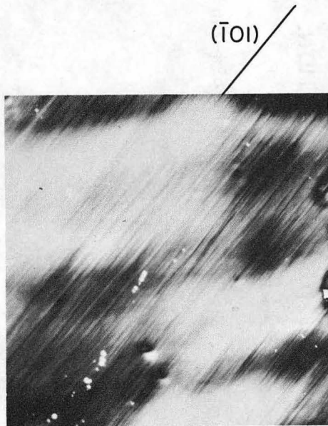
FIG. 11a SLIP TRACES OF SPECIMEN (D2S) DEFORMED AT 77°K TO 0.46% ELONGATION. X'_1 = +16^\circ "D"
