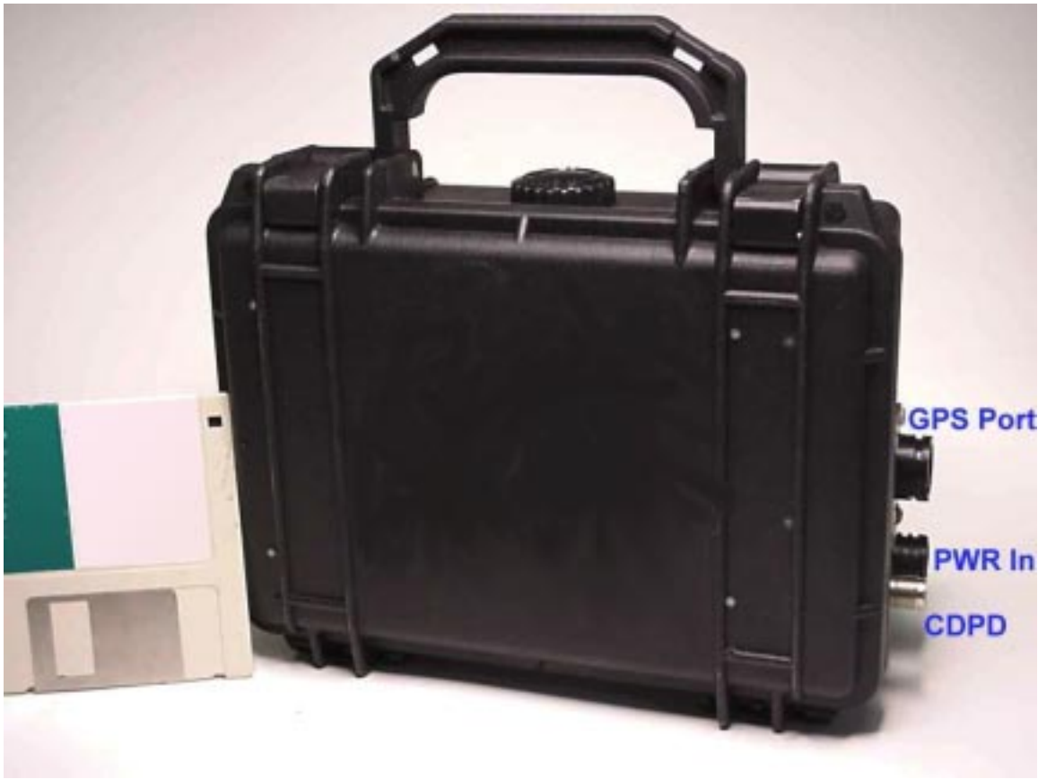
Figure 1. Prototype EDCU in R100 Case (exterior view)
