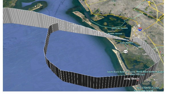
Figure 2. 4D trajectory visualization of go-around flight
