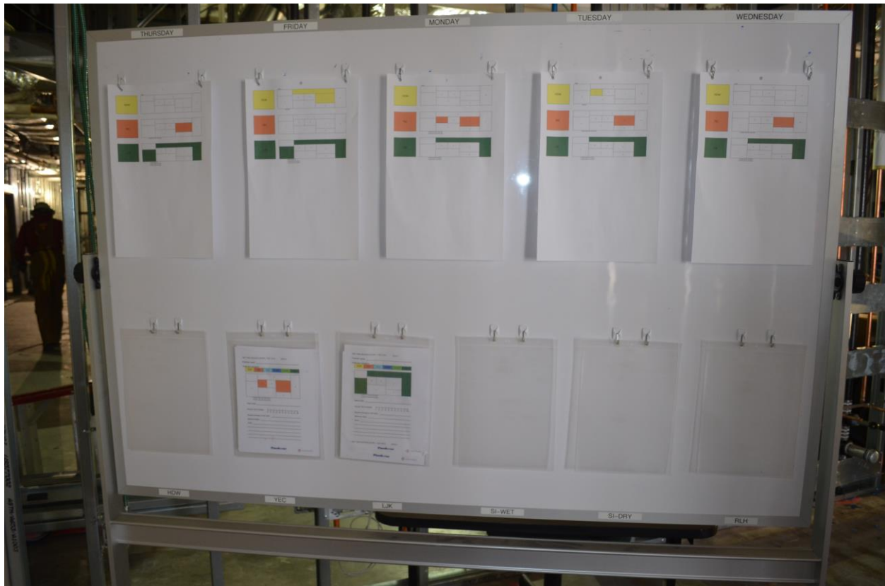
Figure 5-21 – Example of field board showing daily plan; Appendix 1 provides more detail regarding what was shown and how these sheets were automatically generated
