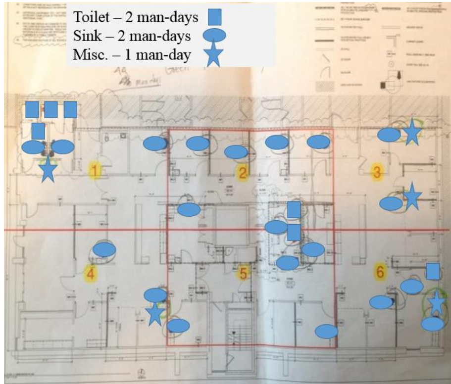
Figure 5-8 – Plumbing inwall rough installation work
