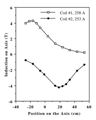
Figure 3. Magnetic Induction on Axis for Individual Coils as a Function of Distance along the Axis and the Coil Current
