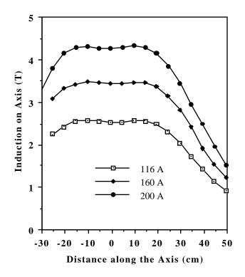
Fig. 4. Magnetic Induction on Axis when the Magnet is Operated in the Solenoid Mode (Coils at the Same Polarity) as a Function of Distance along the Axis and Magnet Current
