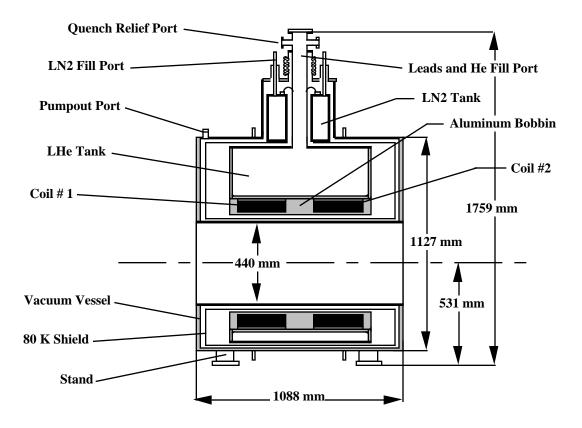
Figure 1. A Cross-section of the RF Test Solenoid and its Cryostat (Note, the magnet and cryostat are eccentric.)
