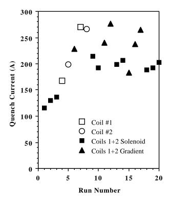
Figure 2. A Quench History for the RF Test Solenoid This history shows the quench current for each magnet run.
