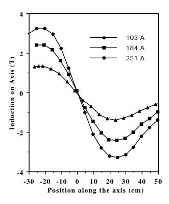
Fig. 5. Magnetic Induction on Axis when the Magnet is Operated in the Solenoid Mode (Coils at Opposite Polarity) as a Function of Distance along the Axis and Magnet Current
