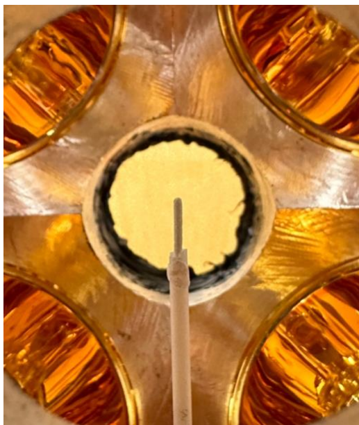
Figure 12: Photo of a sample held using an \text{Al}_2\text{O}_3 tube and ceramic paste adhesive.
